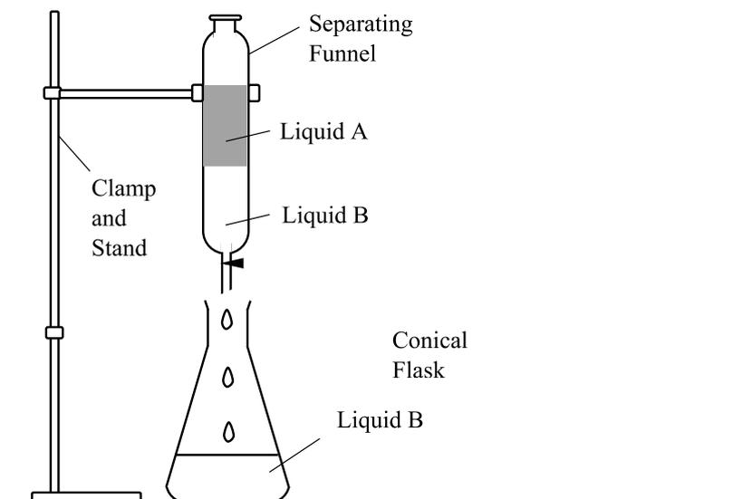
Figure 5: Apparatus diagram for the separation of two immiscible liquids.
