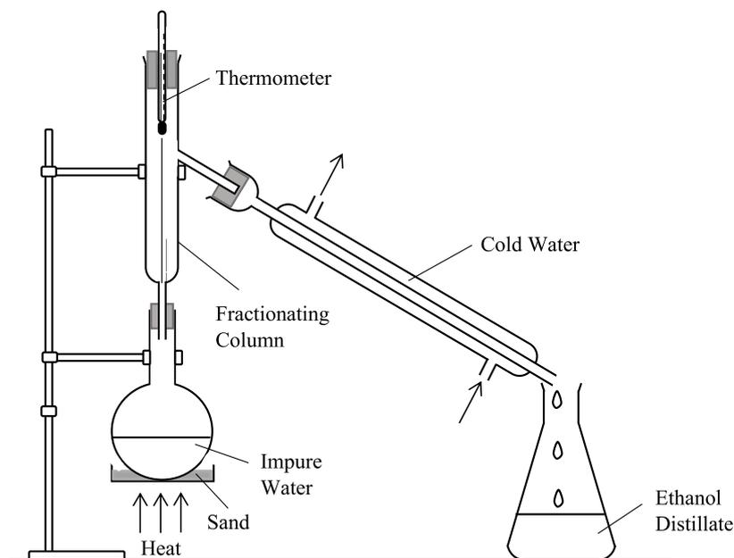
Figure 4: Apparatus diagram for the separation of Miscible liquids.
