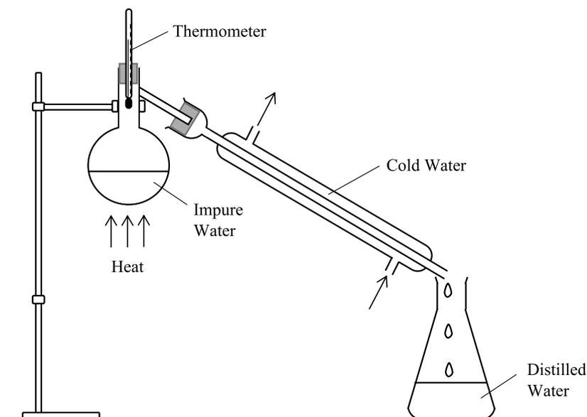
Figure 3: Apparatus diagram for distillation separation technique.
