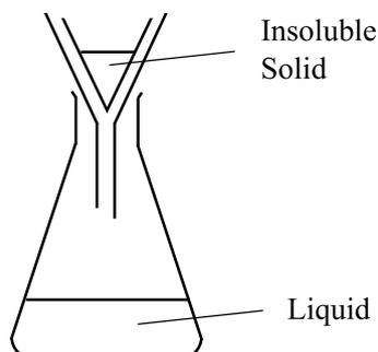
Figure 1: Apparatus diagram for filtration separation technique.
