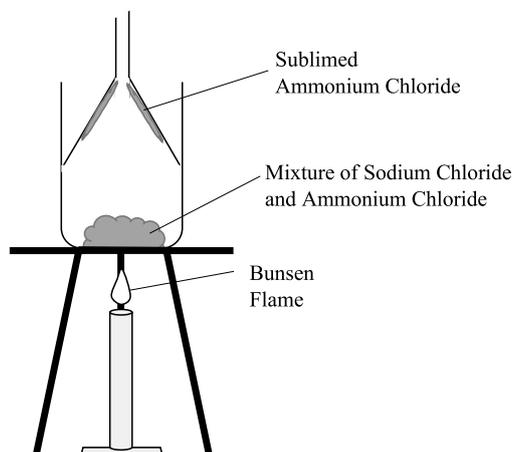
Figure 6: Apparatus diagram the process of separation through sublimation.
