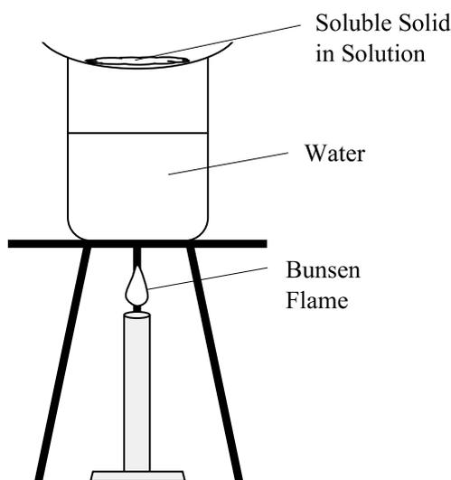
Figure 2: Apparatus diagram for crystallization separation technique.
